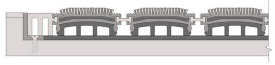
Commence installation with an unshaped mat panel wherever possible, being sure to follow the location indicated in the "Matting order confirmation form". Further panels should then be fitted, ensuring all panels are tight to the divider bars and with no gaps, except for a 1mm tolerance.
